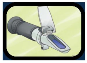
**Step 5**: Use a refractometer, hydrometer, or salinity probe to obtain a specific gravity ideally between 1.021 and 1.025.
